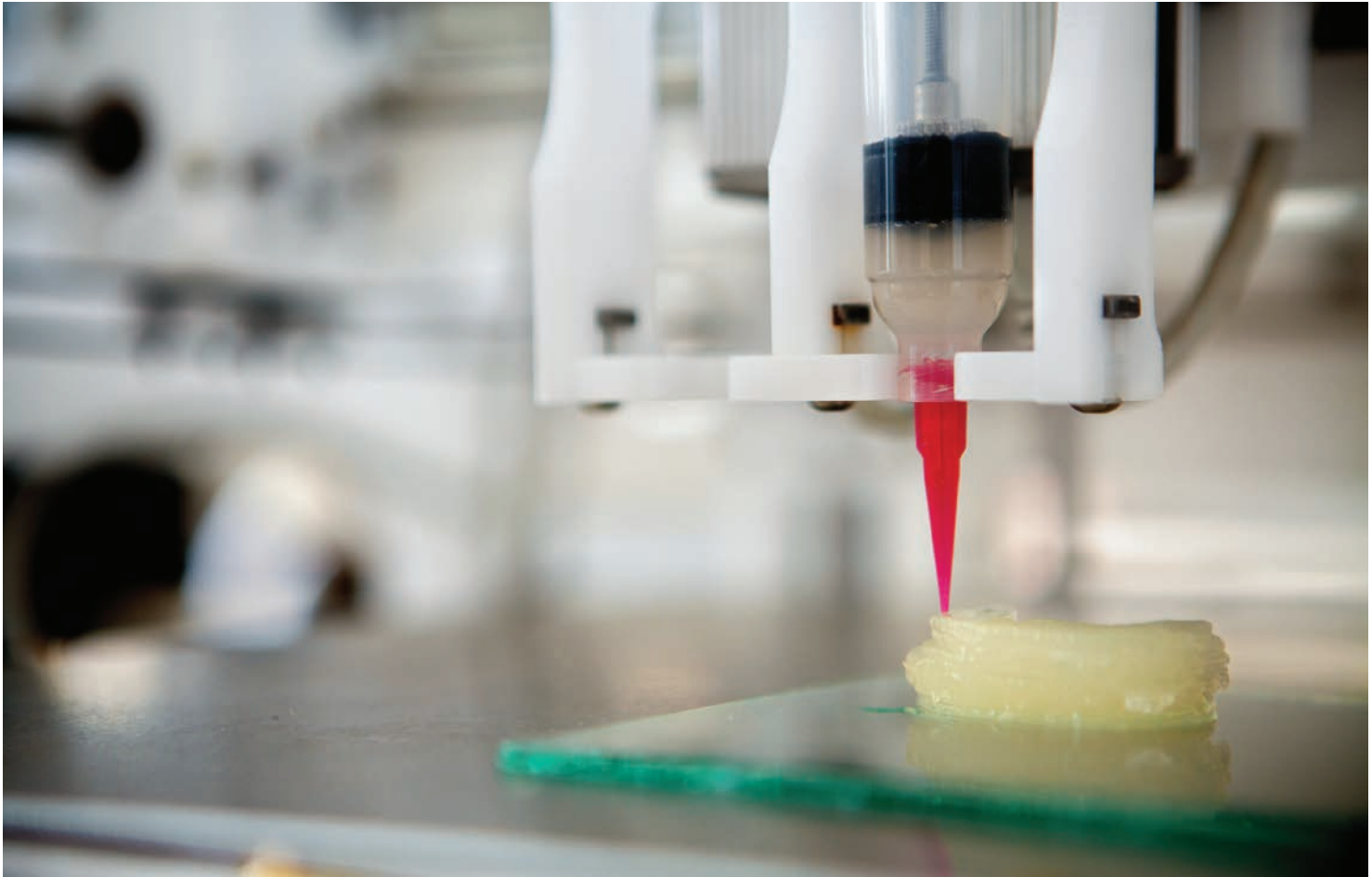
Hear, hear: In the Ithaca lab of Larry Bonassar, PhD (right), a 3-D printer forms an artificial ear (above).
